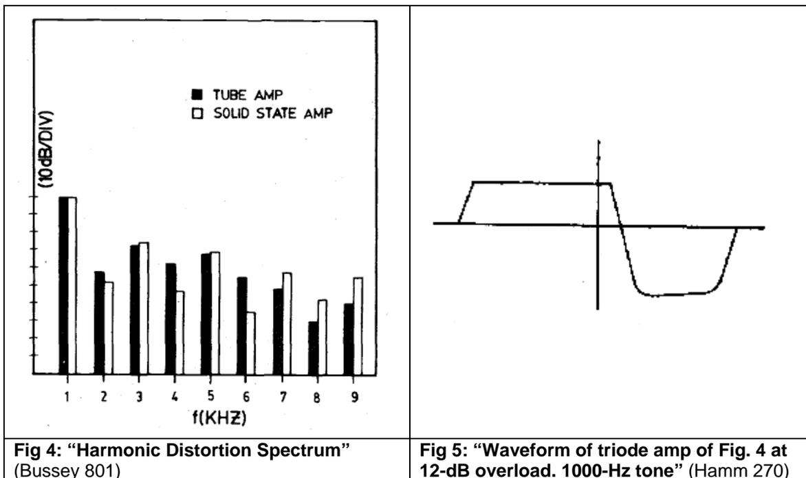
Their results are consistent with Hamm’s findings, showing that tube amplifiers favor even order harmonics, while solid state (transistor) amplifiers with the same one hundred
