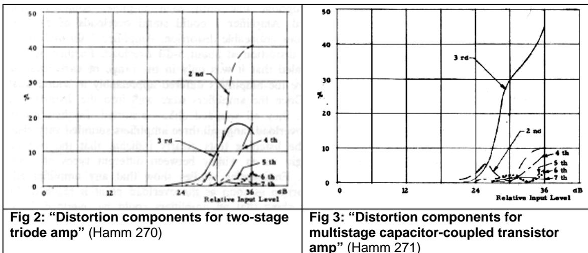
A careful analysis of these graphs demonstrates that the tube amplifier emphasizes the second order harmonic while the transistor amplifier has a substantial third order harmonic. Hamm describes the even order harmonics (such as the second) as adding a
