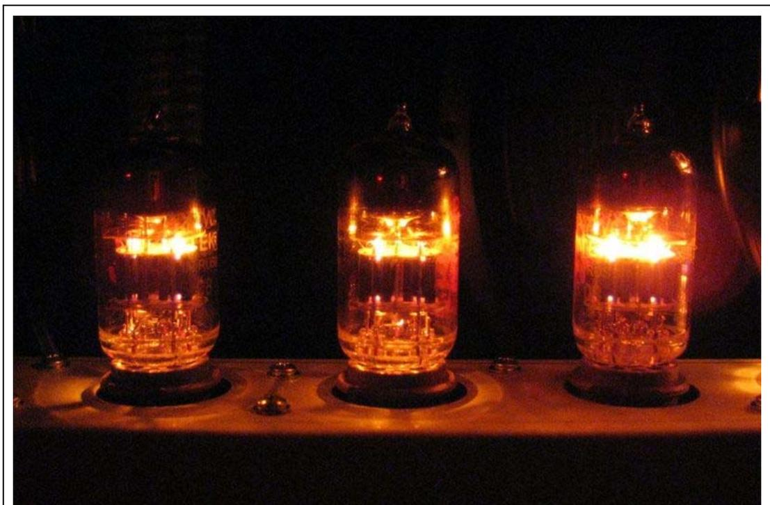
**Fig 1: Three 12AX7 Vacuum Tubes, commonly used in Guitar Amplifier Preamps**
